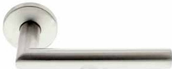
4204.19.SS Straight mitred, Ø19mm round bar lever handle on rose with bolt through fixings at 38mm centres.
