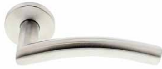
4205.19.SS Curved mitred Ø19mm round bar lever handle on rose with bolt through fixings at 38mm centres.
