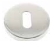
Product Ref: 4213.8.SS 4214.8.SS 4215.8.SS Function: Euro profile cylinder escutcheon Lever key escutcheon Blank escutcheon Description: Ø52 x 8mm with snap on cover. Supplied as pairs as standard. Bolt through fixings supplied as standard suitable for doors 44mm-54mm. Alternative fixings available.
