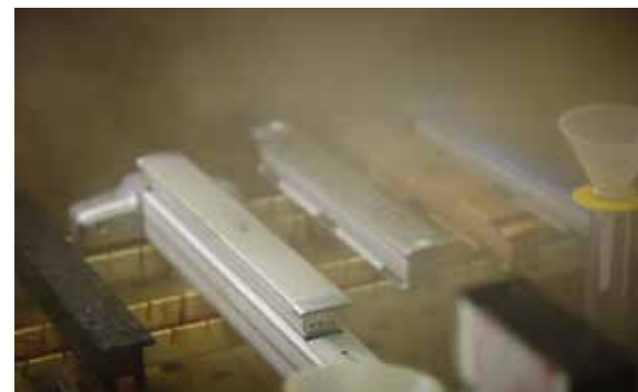
Salt spray corrosion tests being carried out on Von Duprin exit devices.
