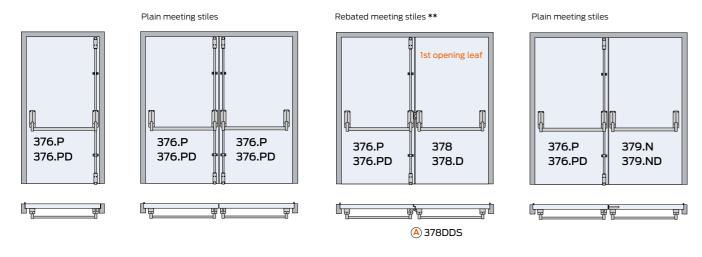
\*\* Consideration should be given to the use of door co-ordinating devices for rebated pairs of doors.
