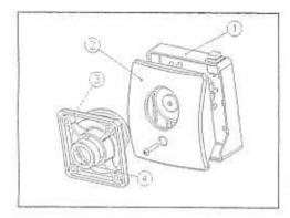
Fit the magnet box (1) to the wall or fixed surface, Check that the screw fixings and the
