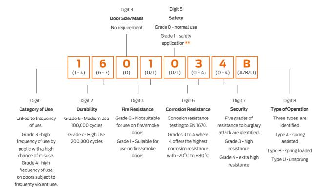
\*\* to qualify for Grade 1 Safety, handles must have high strength lever to plate/rose fixing, high strength plate/rose to door fixing and high strength lever to spindle fixing, such that they would withstand a person grabbing the lever in order to prevent falling.
